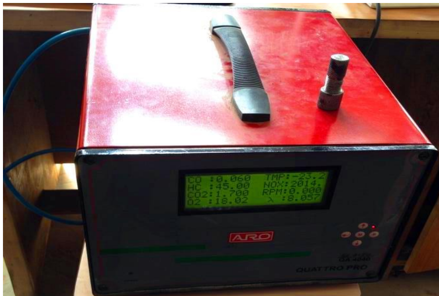
Fig.4. Photographic view of exhaust gas analyzer
