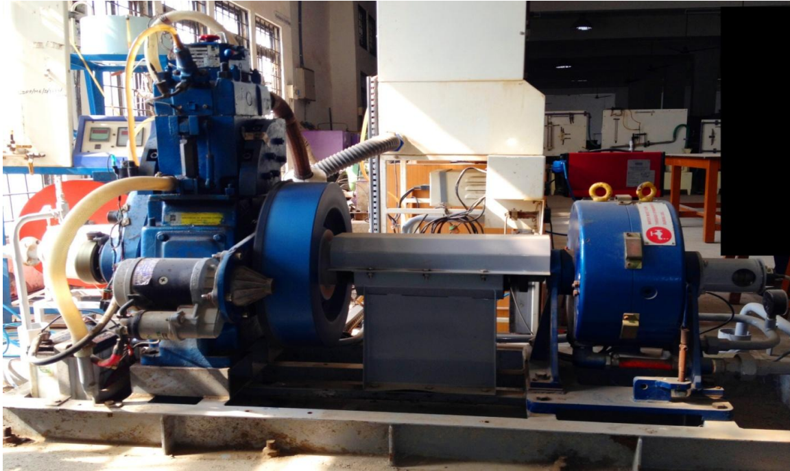
Fig.3 Photographic view of single cylinder four stroke diesel engine
